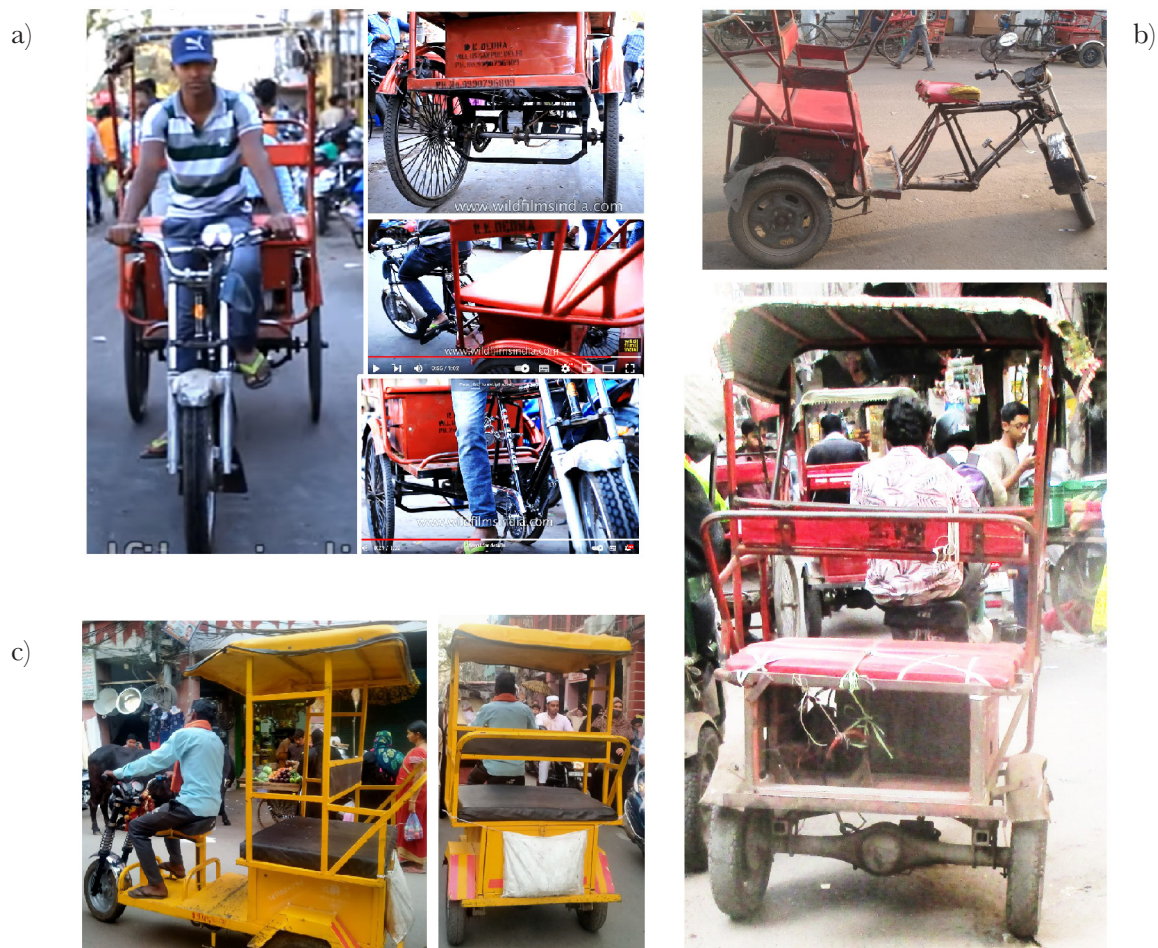
Fig. 3 — Three generations of battery-jugaad from 2014 to 2023. (3a Screen Grab from Youtube Video (Top Left) 60 ; b) (Top and Bottom Right) and c) (Bottom Left) Photographs by the authors.)
