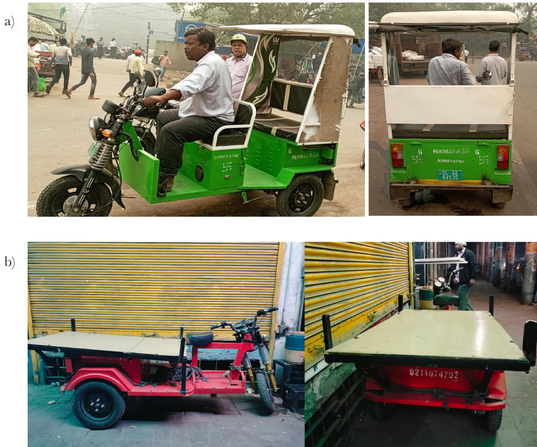
Fig 4 — a) Battery-jugaad , which are registered with transport authorities (Top Left and Right); b) Further transformation of battery-jugaad as a goods vehicle (Bottom Left and Right). Photographs by the authors.
