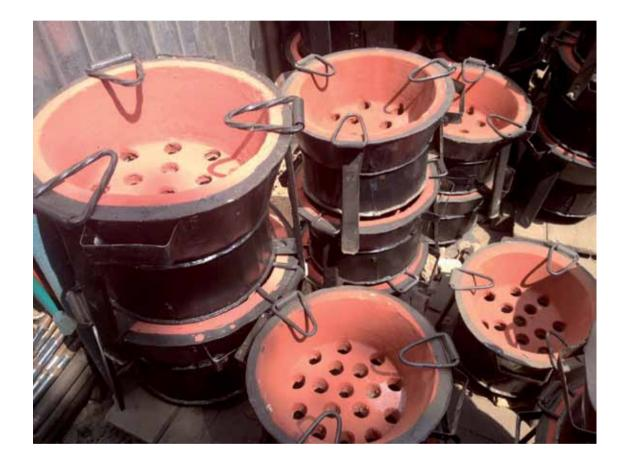
The picture above features a selection of cooking stoves that are produced and sold in the informal metal sector of Nairobi, Kenya. By means of incremental innovation, the cooking stoves have been ingeniously improved by placing a ceramic lining on the inside of the stoves, guaranteeing more efficient use of heat and a reduction in the amount of charcoal used.
